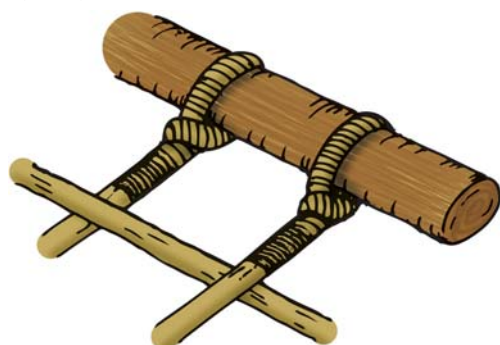
Detail of bedframe in which the straps supporting the mattress are tied over the bedframe
