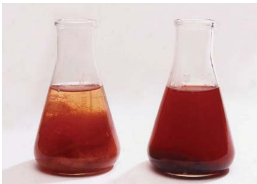
Left: Boiled solution after wool has been added (orange). Right: Boiled solution with Kermes echinatus (red).
