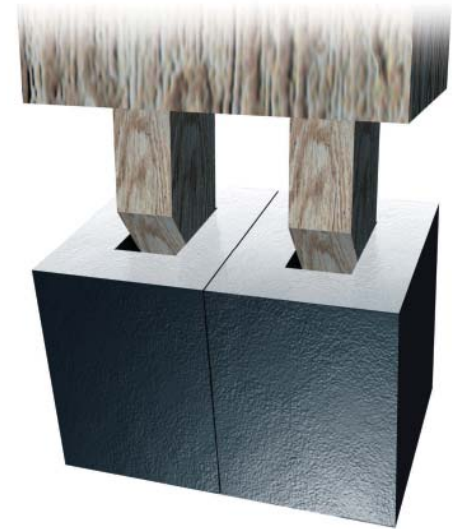
Bottom of beam fitting into socket
