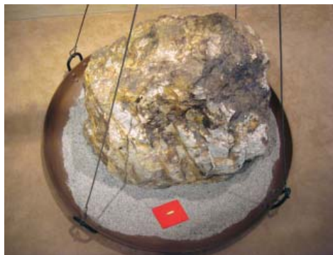
Gold ore from the Toi gold mine in Japan. After extraction, an 860 kg rock such as this one yields 30 g of gold, as seen on the red square.
